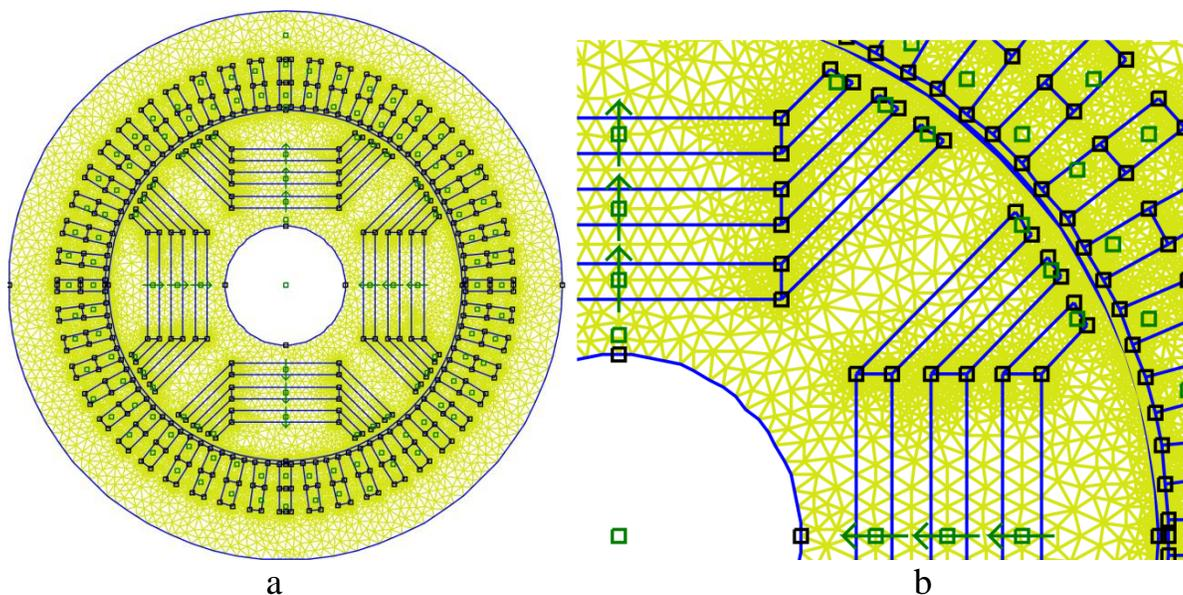
Fig. 3 Finite element mesh of a synchronous jet engine with sectioned permanent magnets: a – general view; b – permanent magnet zone
