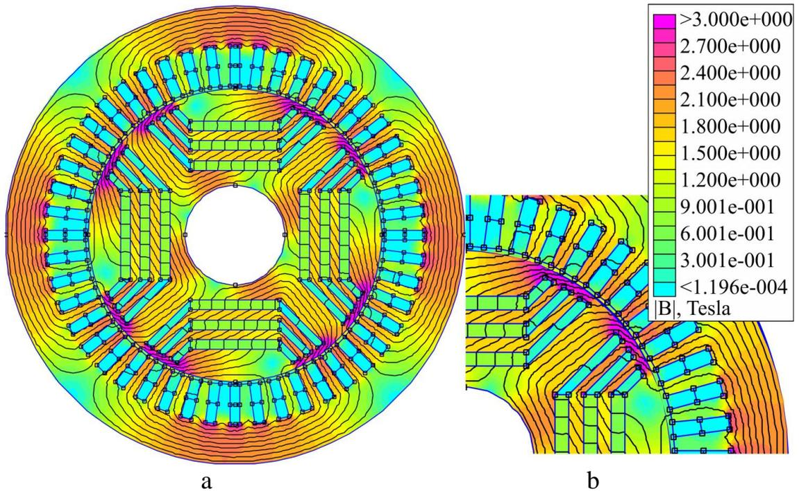
Fig. 5 Results of calculation of the magnetic field of a synchronous jet motor with sectioned permanent magnets in nominal mode: a – general view; b – zone of permanent magnets
