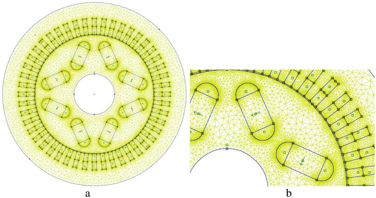
Fig. 2 Finite element mesh of a synchronous jet motor with non-sectioned permanent magnets: a – general view; b – permanent magnet zone
