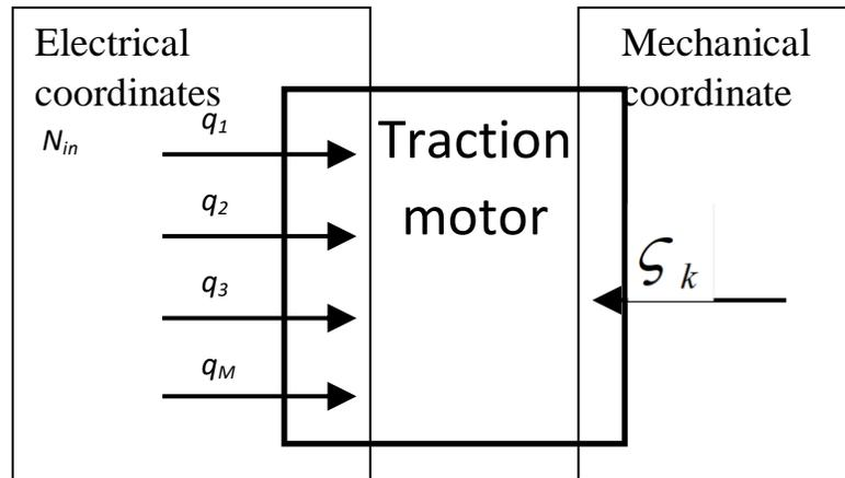
Fig. 1 – Structural diagram of the mathematical model of a traction motor
