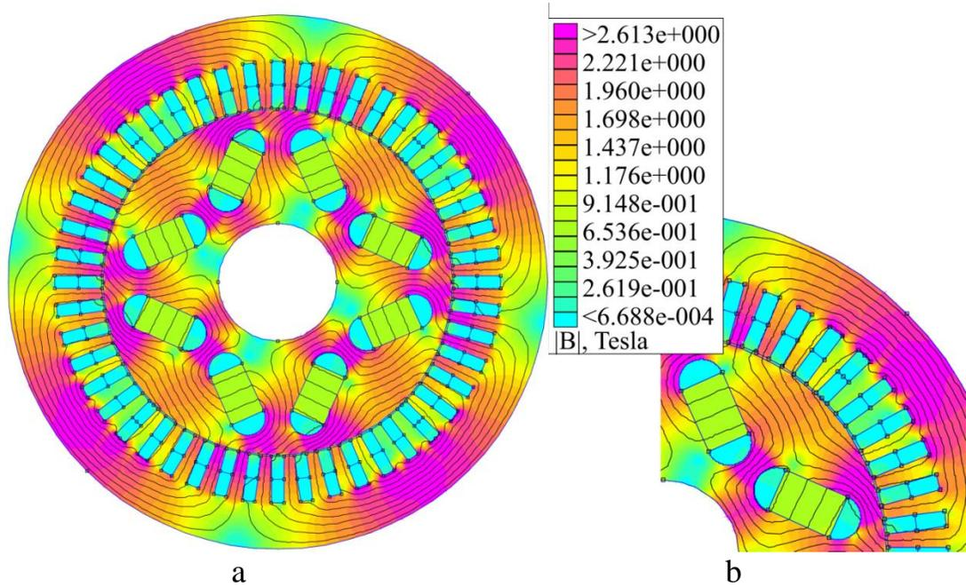
Fig. 4 Results of calculation of the magnetic field of a synchronous jet motor with non-sectioned permanent magnets in nominal mode: a – general view; b – zone of permanent magnets.
