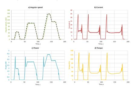
Fig. 2. Sample urban driving cycle ECE-R15 applied to the loaded testing motor
