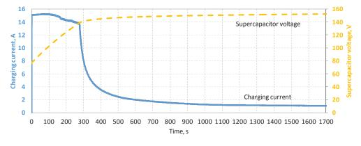
Fig. 4. Voltage and current responses obtained during the supercapacitor charging
