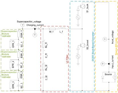
Fig. 3. PSIM simulation scheme of the supercapacitor bench
